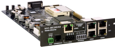
FIG. 1 NXC-ME260/64 Master Card (front view)
